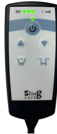
Handset 5 button handset for motors' activation
